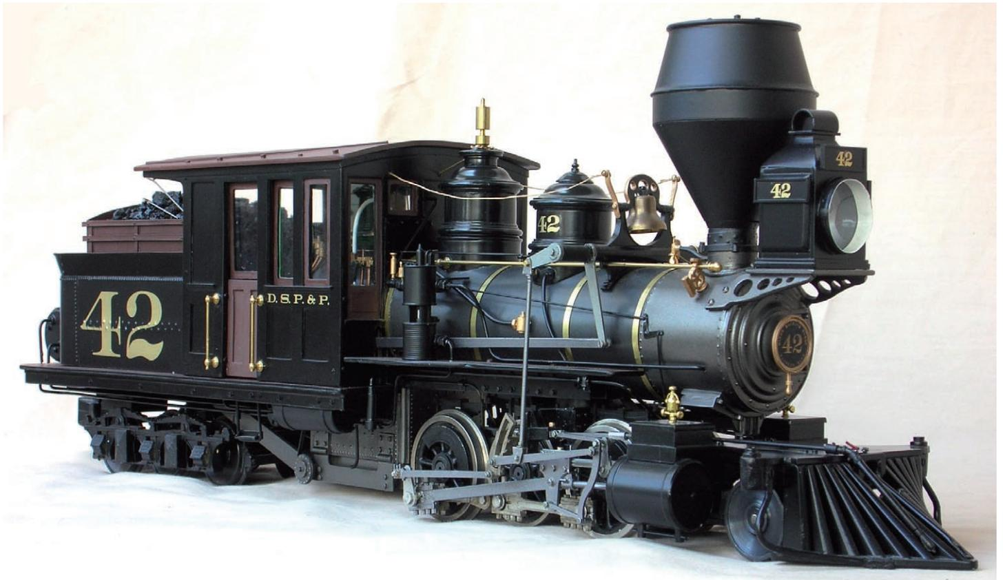
The chassis was a custom designed effort via 'Barrys Big Trains' in Arizona, and features cast magnesium main rod and side rods, cast from CNC machined masters developed in 3D cad, and finally a laser cut stainless steel valve gear set, cut here in Melbourne.
