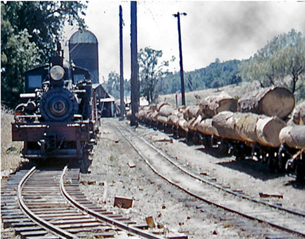
We got this close to the to the dump area before turning around to see if another train was coming. Shay no. 9 is about to be uncoupled from the log cars which are lined up along the brow log. Shay no. 15 is in the RIP or dead line at the left.
