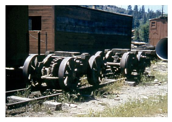
This is a close up of the two Heisler trucks. The tires had been removed and were piled elsewhere.
