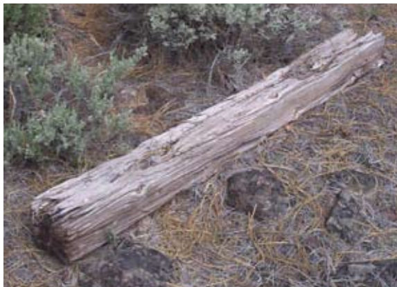
Photo B (above) and Photo C (left): Surviving railroad ties with spikes and spike holes allowed the gauge of the line to be established at 36" between the rails. Photo B: April, 1010, Photo C: June, 2006 by the author.
